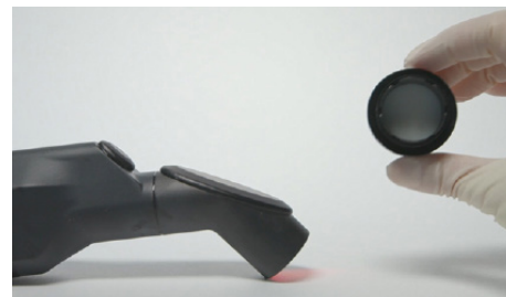
Fig.24. Remove plate from handheld probe
