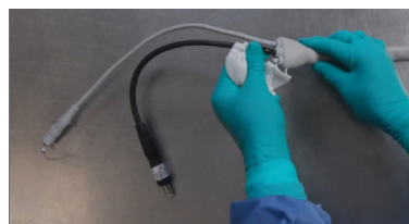
Fig.83. Wipe connector end
