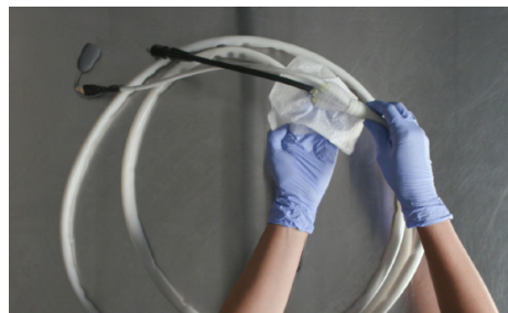
Fig.76. Clean handheld probe and cables
