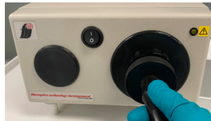
Fig.9. Plug light guide into light source
