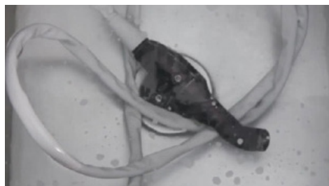
Fig.87. Soak handheld probe and cables
