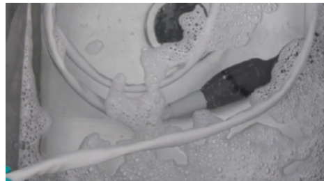
Fig.84. Submerge handheld probe and cables
