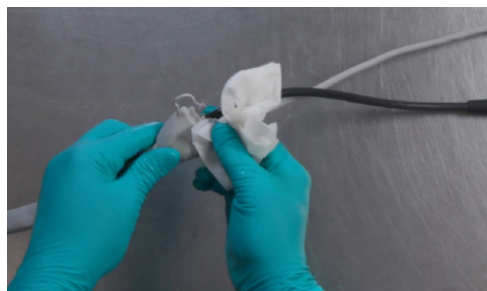
Fig.88. Wipe connector end with RO/DI-soaked cloth
