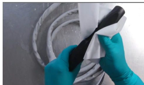
Fig.89. Dry handheld probe and cables
